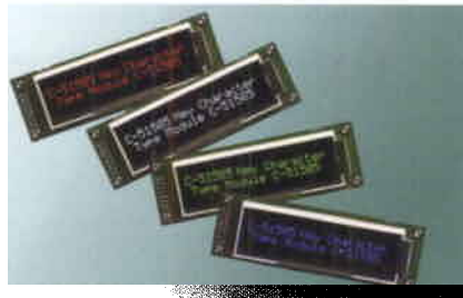
Figure 1. These C-51505 20-character \times 2-line monochrome displays from Optrex offer improved performance in an industry-standard configuration as well as a striking appearance and a range of color options.
